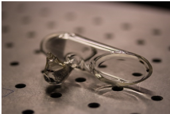
Figure 24: Potassium vapor cell with Brewster angled windows
