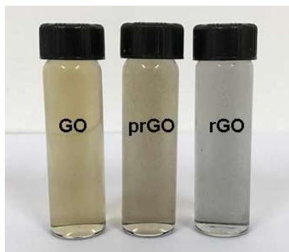
**Figure III.1.2.** Photograph of glass bottles containing water dispersions of graphene oxide (GO), partially reduced graphene oxide (prGO) and reduced graphene oxide (rGO).
